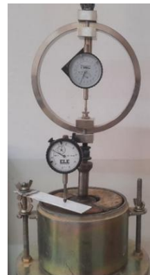
Figure 3. Initial stage of the CBR test (GTX placed between the sand layer and the loading half-discs)
