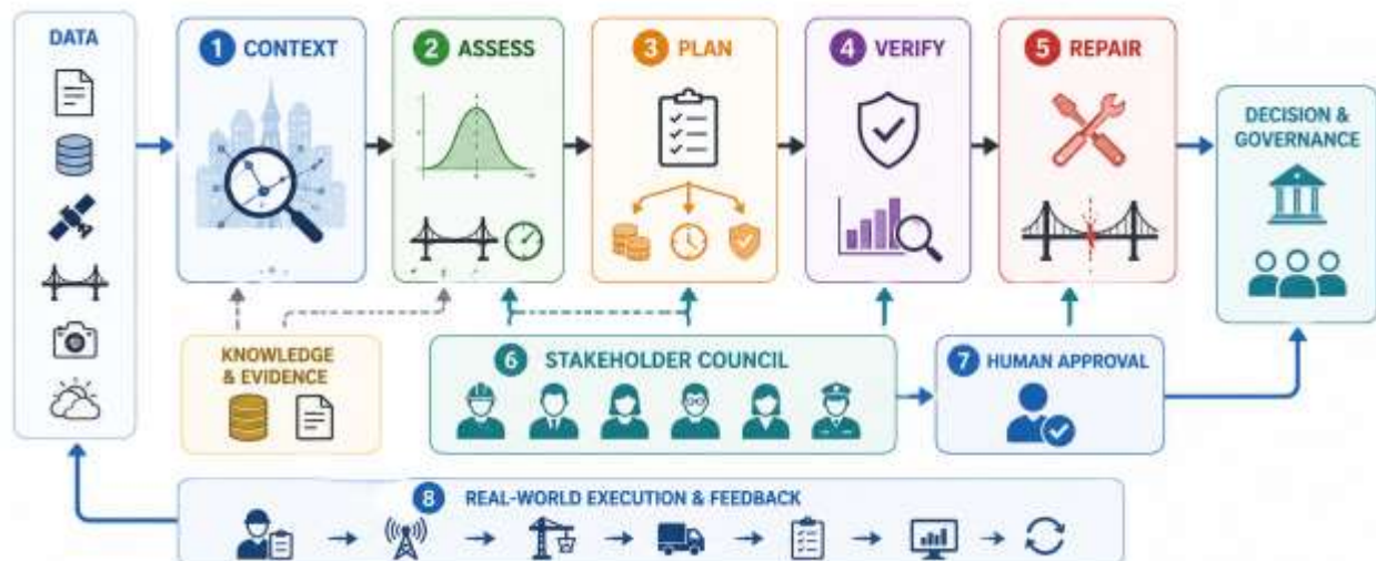
Figure 1. Implemented closed-loop architecture from evidence ingestion to intervention feedback.
