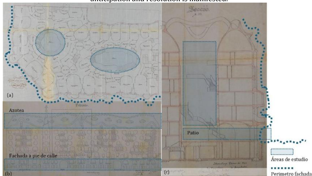
Figure 3. (a) Floor plan of the apartments, (b) exterior elevation, and (c) cross-section of Casa Milà, showing the undulating continuity of pathways and heights, where the perceptual sequence of anticipation and resolution is manifested.
