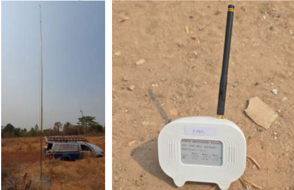
Figure 5. Mobile 14 m gateway pole and sniffer
