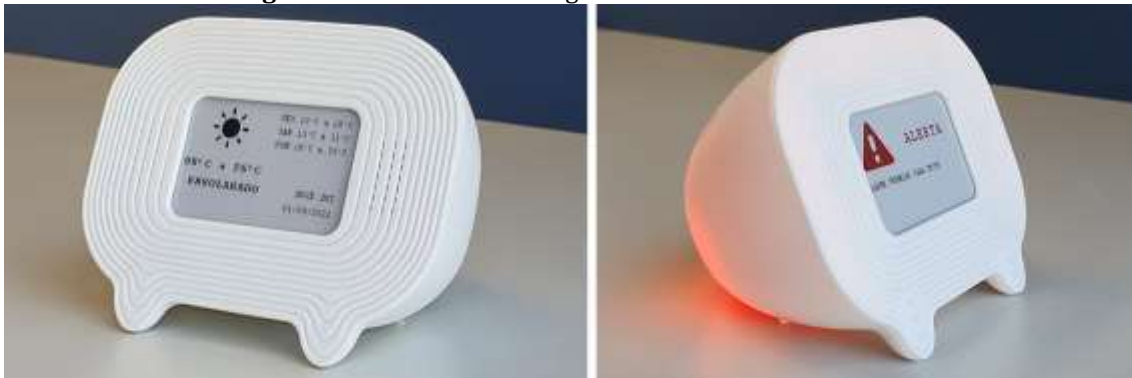
Figure 2. DIN device showing weather forecast and alarm.
