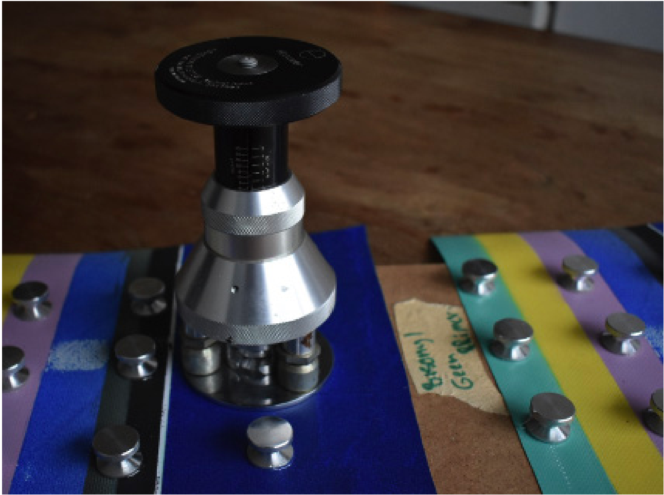
Figure 4: Adhesion test on samples of painted canvases Author: Pieter Keune
